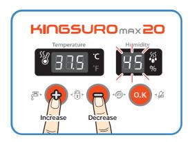
(Tip) If you want to up incubator humidity 0.5%, you should calibrate 0.5% lower in calibration mode.
