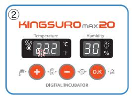
\* The artificial intelligence system memorizes and classifies ambient conditions for keeping optimum temperature, and temperature can move up slowly at the first stage.
